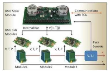
left in the battery (fuel gauging), or it could be used for more advanced control features.
