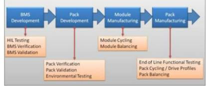
manufacturers are BMS development, pack development, module assembly, and pack assembly. What tests are performed at each step is a different matter altogether, and depends on the specifics of the process and the device.
