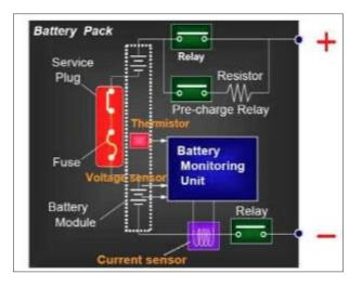
To assist in manufacturing and assembly, the large stack of cells is typically grouped into smaller stacks called modules. Several of these modules will be placed into a single battery pack. Within each module the cells are welded together to complete the electrical path for current flow. Modules can also incorporate cooling mechanisms, temperature monitors, and other devices. In most cases, modules also allow for monitoring the voltage produced by each battery cell in the stack by the BMS.
