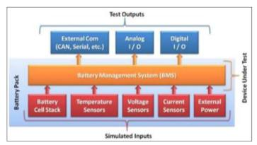
or individual components of the system. Of course your specific requirements will be different, but an example BMS testing solution might have the following physical requirements:
