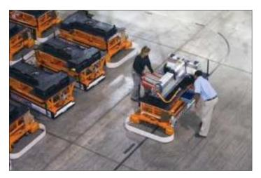
After EOL functional testing is completed, packs may also be subjected to charge / discharge cycling and drive profile cycling, which will simulate the typical conditions the pack will see when integrated into the EV drivetrain. Packs can also be run through active cell balancing routines in order to set the initial charge state of each cell to a nominal condition, or to set the Pack SoC to a level appropriate for shipping and storage.
