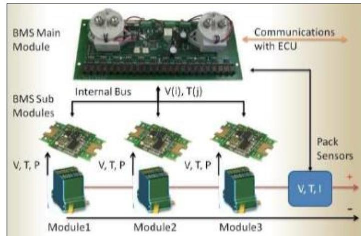
For example, SoC information is critical to estimating and maintaining the pack's usable lifetime. Usable battery life can be dramatically reduced by simply charging the pack too much, or discharging it too deeply. The BMS must maintain the cells within the safe operating limits. The SoC indication is also used to determine the end of the charging and discharging cycles.
