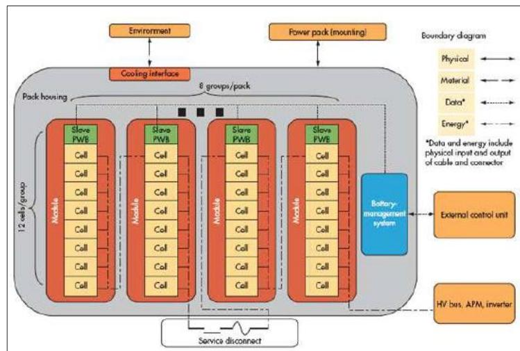
Cell balancing is an active way of compensating for weaker cells by equalizing the charge on all the cells in the chain and thus extending the battery pack's usable life. During cell balancing circuits are enabled which can transfer charge selectively from neighboring cells, or the entire pack, to any undercharged cells detected in the stack.
