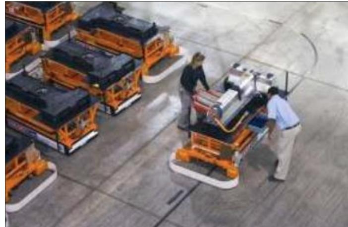
After EOL functional testing is completed, packs may also be subjected to charge / discharge cycling and drive profile cycling, which will simulate the typical conditions the pack will see when integrated into the EV drivetrain. Packs can also be run through active cell balancing routines in order to set the initial charge state of each cell to a nominal condition, or to set the Pack SoC to a level appropriate for shipping and storage.
