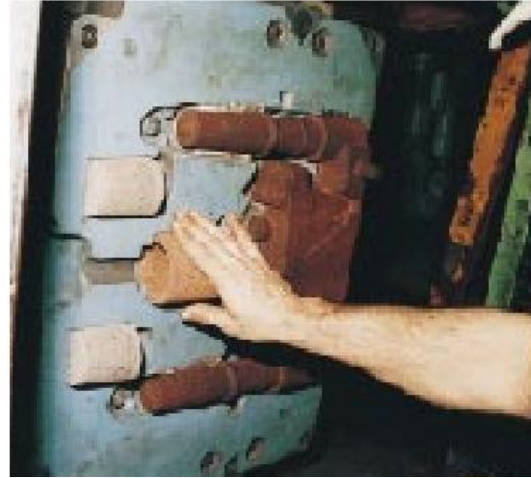
Figure 3. A core is a solid block of molded sand held by a binding agent. It is placed in the Coresetter to form a hollow cavity in the final metal part.
